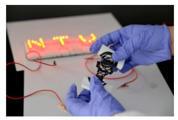
The supercapacitor functions well even when stretched.
