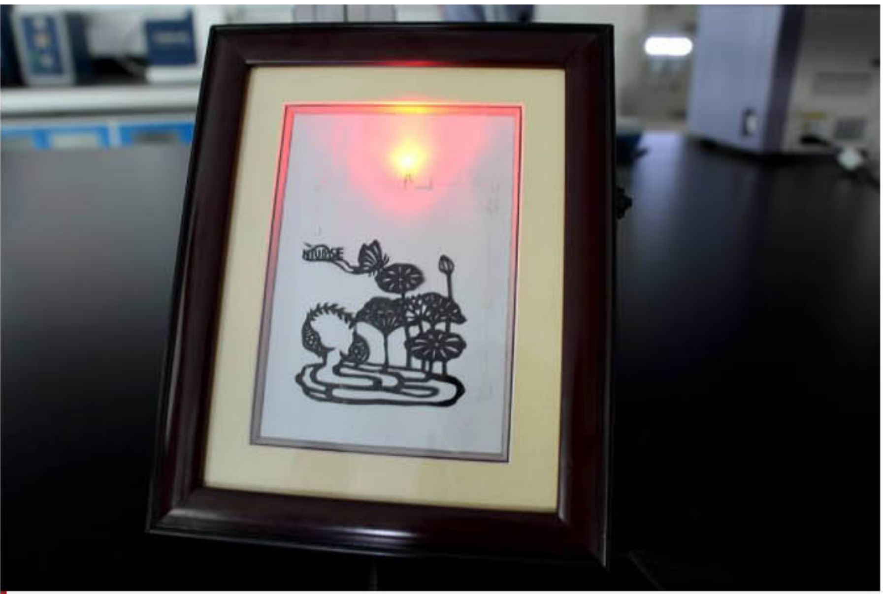
An intricately designed supercapacitor powering a light. Such customisations open up new possibilities for wearable electronics in future. (Photo: NTU)
