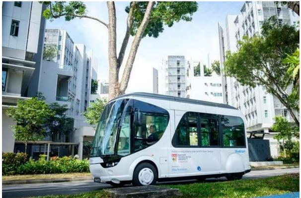
Developed by Blue Solutions, Bolloré Group, the shuttle undergoes quick charging at charging stations, while passengers board or alight (Image credit: Nanyang Technological University)
