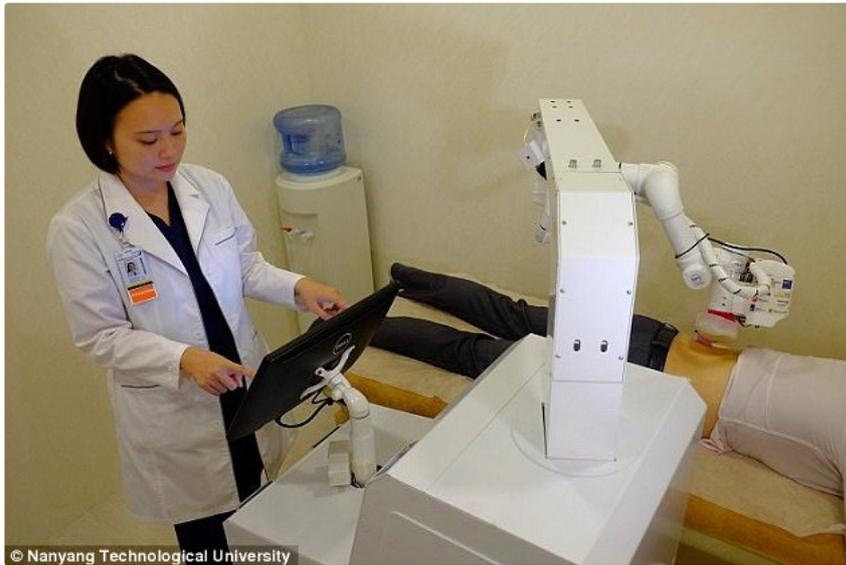
Emma has a touch screen with a fully articulated robotic limb with six degrees of freedom – meaning she can move forwards, backwards, up, down, left and right, and rotate. At the end of the bot are two soft massage tips made of silicon, which can be warmed for comfort
