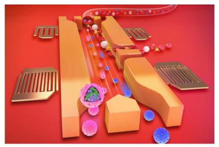
This schematic shows a microfluidic device that uses sound waves to separate exosomes (pink spheres) from other components of blood. Courtesy of Mengxi Wu, Ming Dao, Subra Suresh, Yoel Sadovsky and Tony Jun Huang
