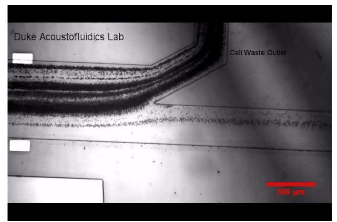
Duke University researchers have developed a prototype device that uses sound waves to separate tiny particles called exosomes from blood samples. Cells produce exosomes to communicate with one another and could play a large role in future diagnostics and therapeutics. Credit: Kara Manke, Duke University
