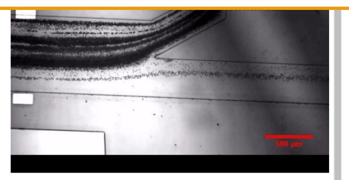
Duke University researchers have developed a prototype device that uses sound waves to separate tiny particles called exosomes from blood samples. Cells produce exosomes to communicate with one another and could play a large role in future diagnostics and therapeutics.
