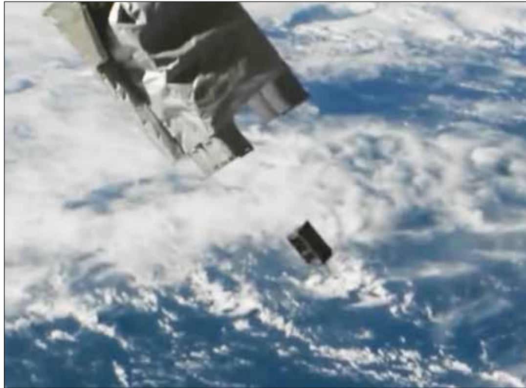
The Aoba Velox-III (bottom) nano-satellite, which weighs 2.3kg, was shot into orbit around the Earth using a special launcher (top) by a Japanese astronaut at the ISS, instead of being launched from a rocket. PHOTO: NTU
