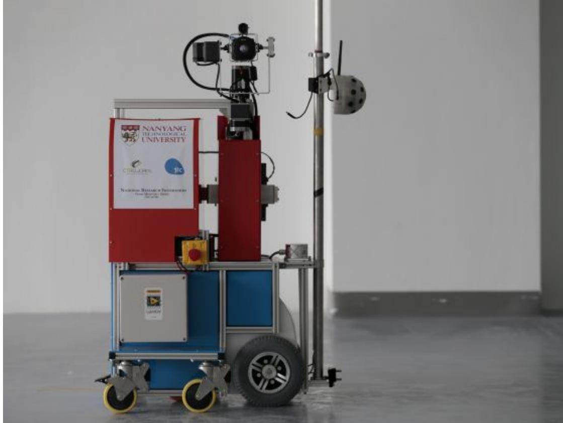
SINGAPORE — Meet QuicaBot, which has a special talent in finding fault. This new robot, invented by a group of four scientists from Nanyang Technological University (NTU), is able to inspect indoor spaces using laser scanners and high-tech cameras, to help detect defects and uneven surfaces faster and more thoroughly than humans.
