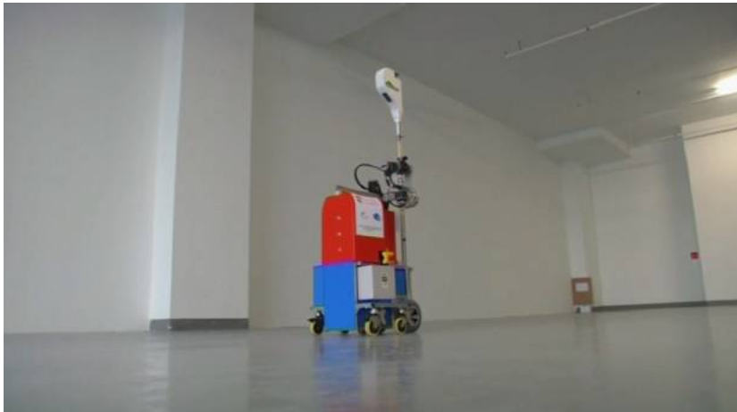
Singapore's Nanyang Technological University developed the QuicaBot, a robot designed to inspect buildings for defects. — Reuters pic
