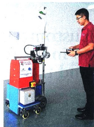
QuicaBot can detect if walls meet at right angles or floors are even. If it takes two human inspectors a day for inspection, JTC estimates that a human inspector and robot pair will take only half a day.
