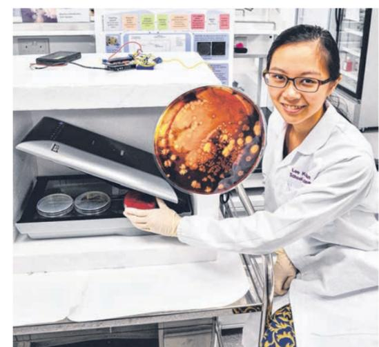
By combining a styrofoam box, heater, fan and scanner, medical student Aletheia Chia built a device that can grow and image bacteria, for under \$400. An incubator sells for \$3,000 while a small imaging system can cost over \$10,000. PHOTOS: NTU, LIM SIN THAI
