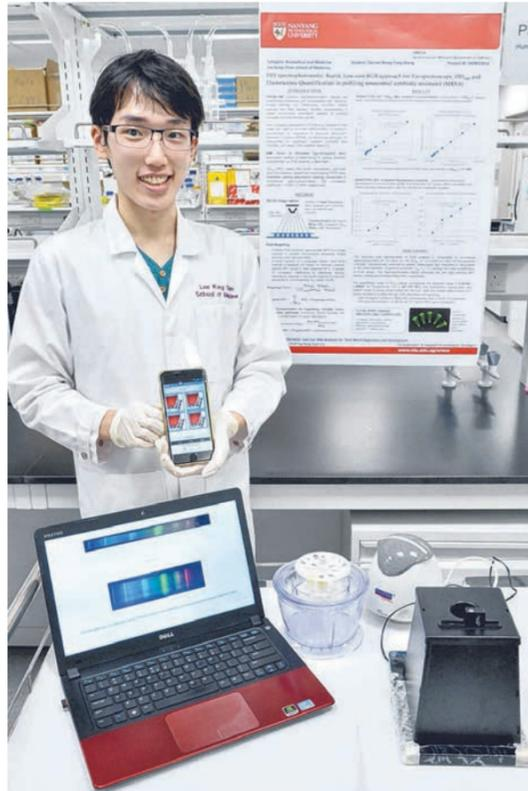
Medical student Darren Wong used a cellphone camera and a DVD disc to develop a portable spectrophotometer for determining antibiotic resistance. Commercial devices go for up to \$2,500; his version cost under \$300.
