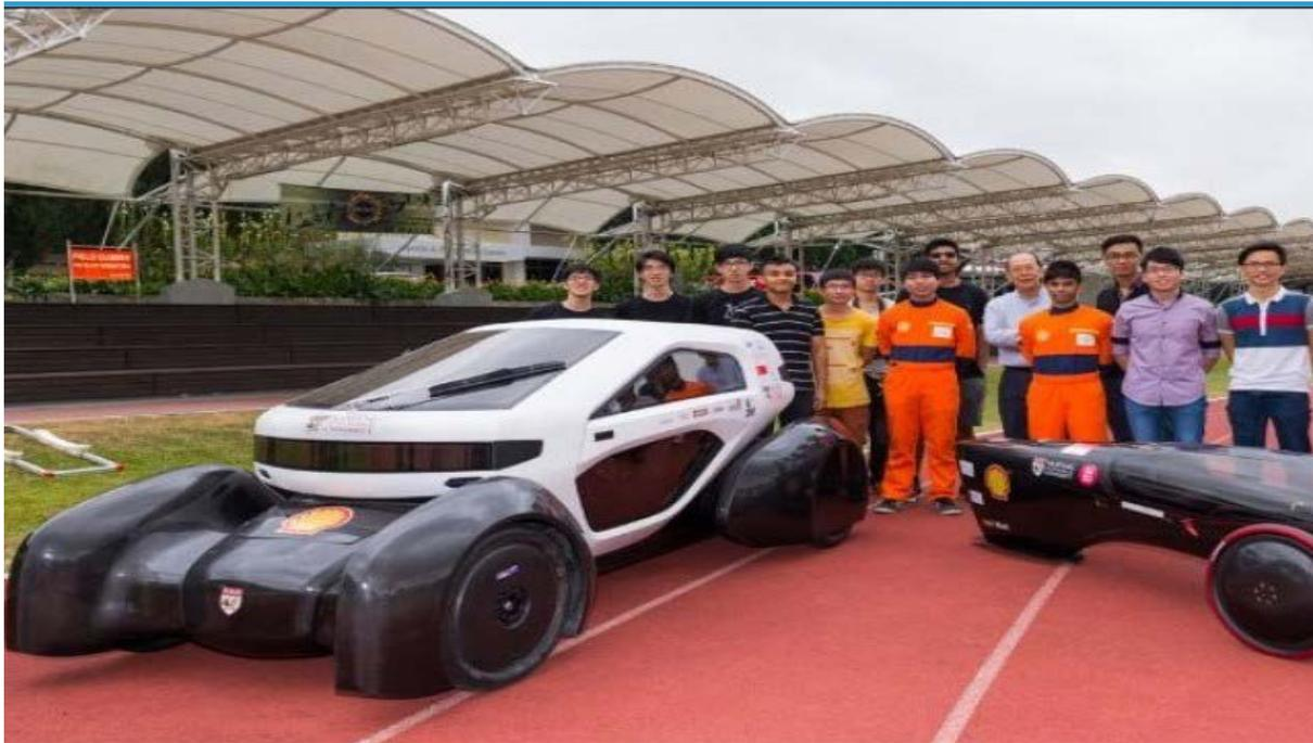
**Students at Nanyang Technological University (NTU) have built a solar powered car with a 3D-printed body.**
