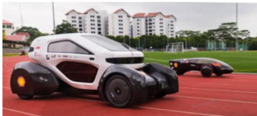
Mounted on a carbon fiber monocoque chassis, the body, internal trim and other components of the NV8 were assembled from 150 acrylonitrile-butadiene-styrene (ABS) parts in ivory and other colors printed on Stratasys Dimension Elite and Fortus 400MC 3D printers.
