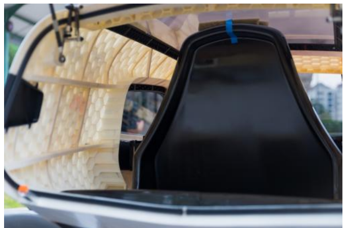
Unique honeycomb design for NV 8 -- Singapore's first Urban Concept car with a 3-D printed body shell. Credit: NTU Singapore
