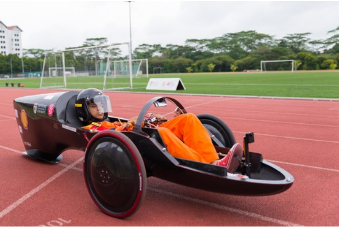
The NV9, an electric racecar whose aerodynamic design is inspired by motorcycles. The car has the ability to tilt, which allows it to navigate corners at high speeds.
