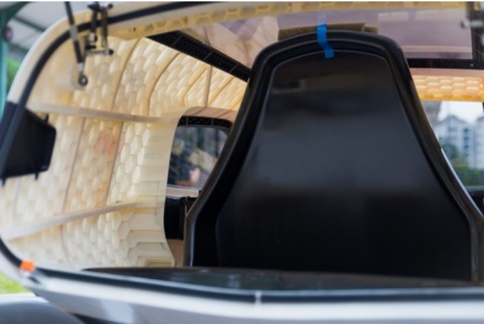
The NV8's unique honeycomb design, which provides structural strength while keeping the weight to a minimum.
