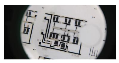
Resistors, transistors and capacitors, the key components of a complex electronic circuit, are printed using non-toxic organic materials like silver nanoparticles, carbon and plastics.
