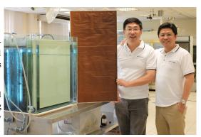
Developed by NTU start-up **Nano Sun**, at the centre of this breakthrough multifunction membrane is a patented titanium dioxide nanotechnology. Titanium dioxide nanoparticles are proven to kill bacteria and to break down organic compounds in waste water with the help of sunlight or Ultra Violet (UV) rays.
