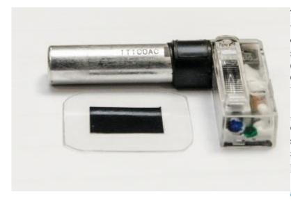
This shows a mobile phone flash unit with its existing capacitor (silver cylinder) compared with NTU's new super thin polymer capacitor material (which is the black colour material). Credit: Nanyang Technological University
